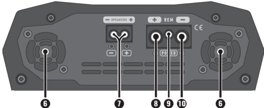
**6. COOLER:** It provides cooling of the amplifier. Install in a cool place without obstruction of air inlets and outlets.
