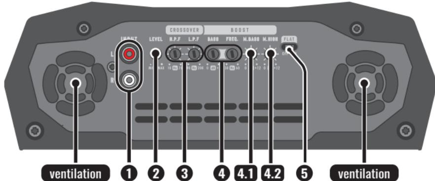
**1. INPUT:** Input of the signal to be amplified. Connect to the radio/player through high quality shielded RCA cables to prevent unwanted noise.
