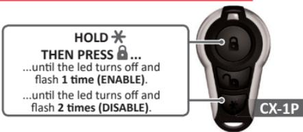
After use, it is recommended that the periodic transmission be disabled to extend **CR2032** battery life (It is recommended that the battery be replaced every 4 months). When the ignition is turned on, the alarm will give 1 beep if the control battery is low.
