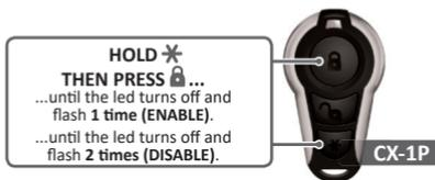
**⚠** After use, it is recommended that the periodic transmission be disabled to extend **CR2032** battery life (It is recommended that the battery be replaced every 4 months). When the ignition is turned on, the alarm will give 1 beep if the control battery is low.
